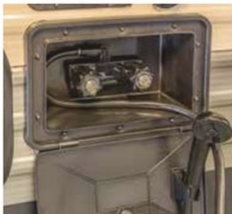
Outside Shower with Hot and Cold Water
