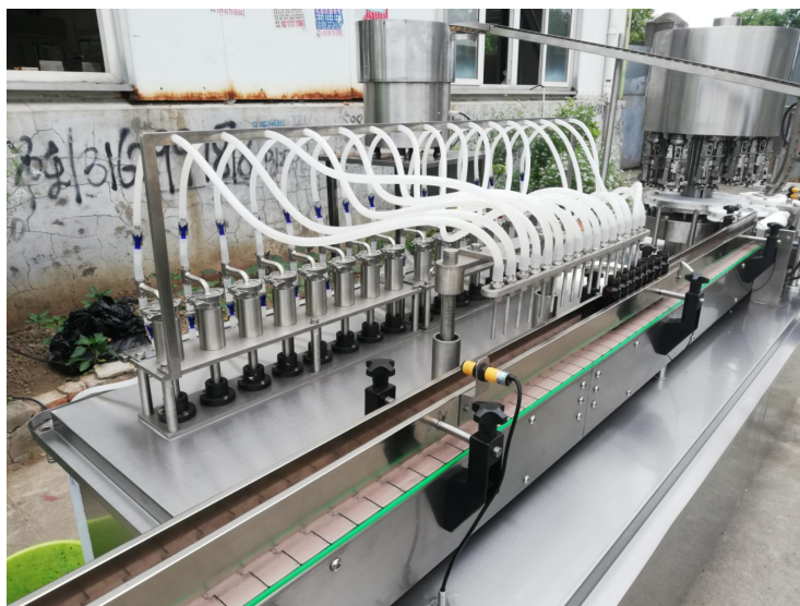
12/ 16 Filling heads, plunger metering pump ,1 add caps,10 screw capping
